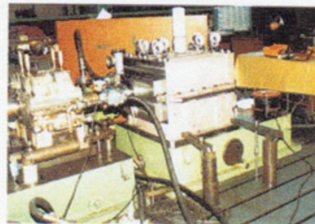
Spur-gear transmission for balancing plant during trials
