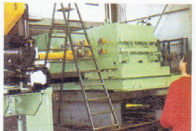
Spur- gear transmission for a steel-sheet straightening machine during a test run
