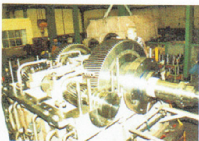
Spur-gear change-speed transmission for balancing plant during assembly
