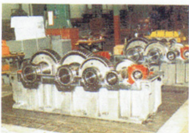
Spur-gear transmission for a briquetting machine during assembly
