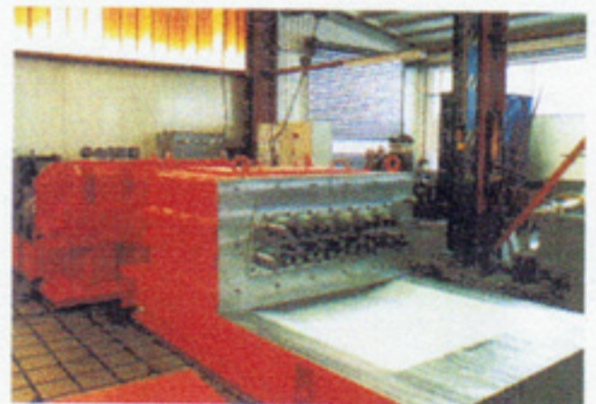
Drive for a steel-sheet straightening machine during a test run
